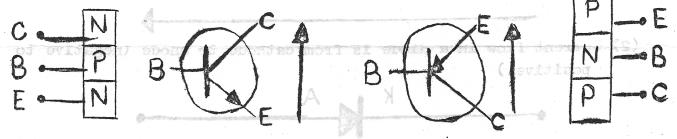
(7) Most NPN transistors are silicom devices, whereas most PNP transistors are germanium devices. The term MOST is not to be confused with the term ALL.
